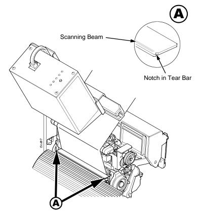
Figure 11. Aligning the Scanning Beam: Continuous, Tear-Off, and Tear-Off Strip Media Handling Modes Only
